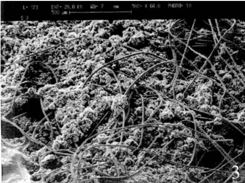
Active charcoal layer of Mxxxx filter. In fig 3 some micro fibres of the outer layer are sticking to the charcoal layer
